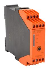
Dold safety relay extension module, on delay, 1 to 10 seconds, 24 VAC/VDC, (3) N.O. time delay and (1) N.C. time delay safety output(s), (1) N.C. time delay monitoring output(s), fixed screw terminals.
