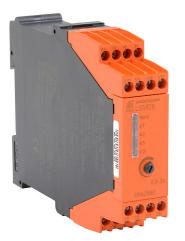
Dold safety relay, emergency stop and safety gates, release delay, 0.3 to 3 seconds, 2-channel, 24 VDC, (2) N.O. and (1) N.O. time delay safety output(s), fixed screw terminals.
