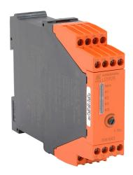
Dold safety relay, emergency stop and safety gates, release delay, 1 to 10 seconds, 2-channel, 24 VDC, (2) N.O. and (1) N.O. time delay safety output(s), fixed screw terminals.
