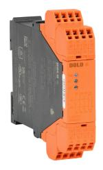
Dold safety relay, emergency stop, safety gate monitoring, 2-channel, 110 VAC, (3) N.O. safety output(s), (1) N.C. monitoring output(s), push-in cage clamp.
