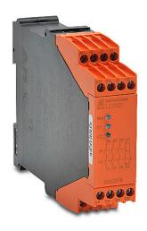
Dold safety relay, light curtain controller, 2-channel, 24 VDC, (3) N.O. safety output(s), (1) N.C. monitoring output(s), fixed screw terminals.
