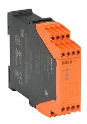
Dold safety relay, emergency stop and safety gates, 2-channel, 24 VAC/VDC, (3) N.O. safety output(s), (1) N.C. monitoring output(s), fixed screw terminals.
