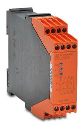
Dold safety relay, emergency stop and safety gates, 2-channel, 110 VAC, (3) N.O. safety output(s), (1) N.C. monitoring output(s), fixed screw terminals.
