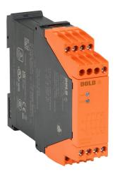
Dold safety relay, emergency stop, 1-channel, 230 VAC, (3) N.O. safety output(s), (1) N.C. monitoring output(s), fixed screw terminals.
