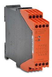
Dold safety relay, emergency stop, 1-channel, 110 VAC, (3) N.O. safety output(s), (1) N.C. monitoring output(s), fixed screw terminals.
