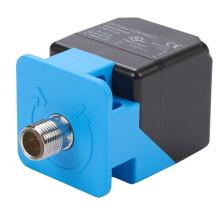
AutomationDirect inductive proximity sensor, rectangular, 40 x 40 x 66mm body, die-cast zinc nickel-plated housing, PNP, N.O. output, 35mm sensing distance, non-flush, 80 Hz switching frequency, IP67, 4-pin M12 quick-disconnect.
