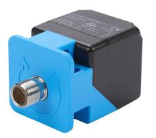
AutomationDirect inductive proximity sensor, rectangular, 40 x 40 x 66mm body, die-cast zinc nickel-plated housing, PNP, N.O. output, 35mm sensing distance, non-flush, 80 Hz switching frequency, IP67, 4-pin M12 quick-disconnect.
