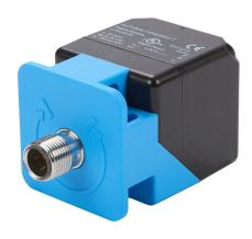
AutomationDirect inductive proximity sensor, rectangular, 40 x 40 x 66mm body, die-cast zinc nickel-plated housing, PNP, N.O. output, 20mm sensing distance, flush, 100 Hz switching frequency, IP67, 4-pin M12 quick-disconnect.
