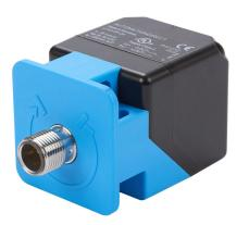
AutomationDirect inductive proximity sensor, rectangular, 40 x 40 x 66mm body, die-cast zinc nickel-plated housing, PNP, N.O./ N.C. complementary outputs, 35mm sensing distance, non-flush, 80 Hz switching frequency, IP67, 4-pin M12 quick-disconnect.
