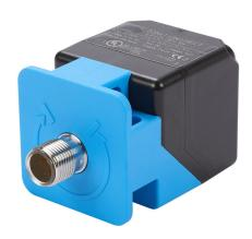
AutomationDirect inductive proximity sensor, rectangular, 40 x 40 x 66mm body, die-cast zinc nickel-plated housing, PNP, N.O./ N.C. complementary outputs, 20mm sensing distance, flush, 100 Hz switching frequency, IP67, 4-pin M12 quick-disconnect.
