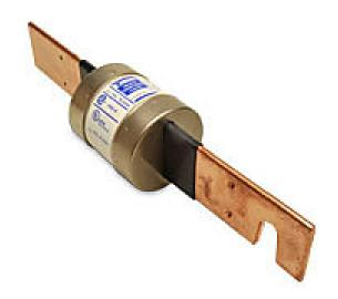
Edison fuse, LESRK series, Class RK1, current-limiting, time-delay, 600A, 600 VAC, knife blade, feeder/branch protection applications.
