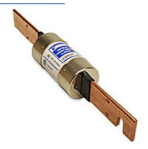
Edison fuse, LESRK series, Class RK1, current-limiting, time-delay, 200A, 600 VAC, knife blade, feeder/branch protection applications.
