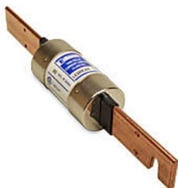
Edison fuse, LESRK series, Class RK1, current-limiting, time-delay, 200A, 600 VAC, knife blade, feeder/branch protection applications.
