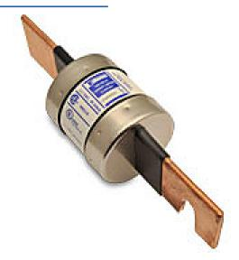
Edison fuse, LENRK series, Class RK1, current-limiting, time-delay, 600A, 250 VAC, knife blade, feeder/branch protection applications.
