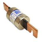
Edison fuse, LENRK series, Class RK1, current-limiting, time-delay, 400A, 250 VAC, knife blade, feeder/branch protection applications.
