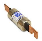
Edison fuse, LENRK series, Class RK1, current-limiting, time-delay, 300A, 250 VAC, knife blade, feeder/branch protection applications.
