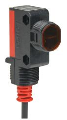
Leuze photoelectric sensor, rectangular, ABS plastic housing, through-beam receiver, 0-10m sensing distance, 10-30 VDC operating voltage, complementary light-on/dark-on, PNP, 4-wire, pigtail.
