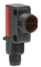
Leuze photoelectric sensor, rectangular, ABS plastic housing, through-beam receiver, 0-10m sensing distance, 10-30 VDC operating voltage, complementary light-on/dark-on, PNP, 4-wire, 4-pin M12 quick-disconnect.
