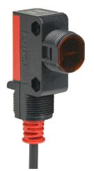
Leuze photoelectric sensor, rectangular, ABS plastic housing, through-beam receiver, 0-10m sensing distance, 10-30 VDC operating voltage, complementary light-on/dark-on, NPN, 4-wire, pigtail.
