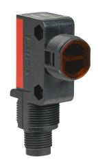
Leuze photoelectric sensor, rectangular, ABS plastic housing, through-beam receiver, 0-10m sensing distance, 10-30 VDC operating voltage, complementary light-on/dark-on, NPN, 4-wire, 4-pin M12 quick-disconnect.
