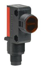
Leuze photoelectric sensor, rectangular, ABS plastic housing, through-beam receiver, 0-10m sensing distance, 10-30 VDC operating voltage, complementary light-on/dark-on, NPN, 4-wire, 4-pin M12 quick-disconnect.
