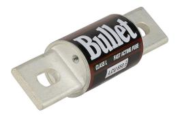
Edison fuse, LCU series, Class L, current-limiting, fast-acting, 650A, 600 VAC, knife blade, feeder/branch, semiconductor protection applications.
