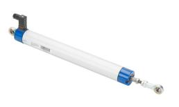
ProSense potentiometer linear position sensor, pivoting slide, 225mm stroke, 38mm diameter x 328mm body, rod eyes mount, 8mm DIN 43650 Form C.
