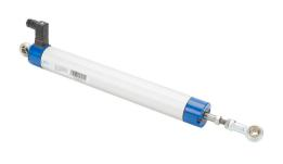
ProSense potentiometer linear position sensor, pivoting slide, 200mm stroke, 38mm diameter x 303mm body, rod eyes mount, 8mm DIN 43650 Form C.
