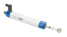
ProSense potentiometer linear position sensor, pivoting slide, 130mm stroke, 38mm diameter x 233mm body, rod eyes mount, 8mm DIN 43650 Form C.
