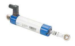
ProSense potentiometer linear position sensor, pivoting slide, 50mm stroke, 38mm diameter x 153mm body, rod eyes mount, 8mm DIN 43650 Form C.
