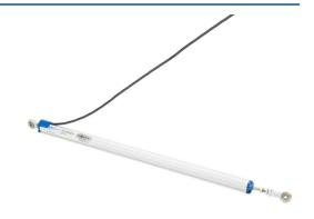
ProSense potentiometer linear position sensor, pivoting slide, 350mm stroke, 18mm diameter x 398mm body, rod eyes mount, pigtail, 3.2ft/1m cable length.
