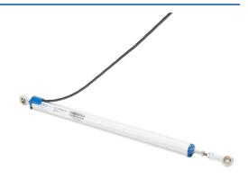
ProSense potentiometer linear position sensor, pivoting slide, 250mm stroke, 18mm diameter x 298mm body, rod eyes mount, pigtail, 3.2ft/1m cable length.
