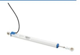
ProSense potentiometer linear position sensor, pivoting slide, 200mm stroke, 18mm diameter x 248mm body, rod eyes mount, pigtail, 3.2ft/1m cable length.
