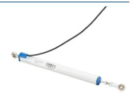
ProSense potentiometer linear position sensor, pivoting slide, 175mm stroke, 18mm diameter x 223mm body, rod eyes mount, pigtail, 3.2ft/1m cable length.
