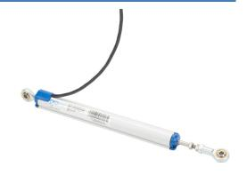
ProSense potentiometer linear position sensor, pivoting slide, 150mm stroke, 18mm diameter x 198mm body, rod eyes mount, pigtail, 3.2ft/1m cable length.
