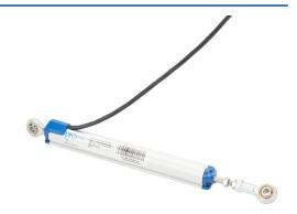
ProSense potentiometer linear position sensor, pivoting slide, 125mm stroke, 18mm diameter x 173mm body, rod eyes mount, pigtail, 3.2ft/1m cable length.
