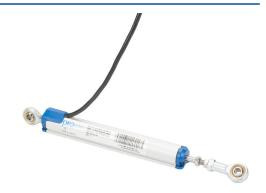
ProSense potentiometer linear position sensor, pivoting slide, 100mm stroke, 18mm diameter x 148mm body, rod eyes mount, pigtail, 3.2ft/1m cable length.
