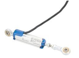
ProSense potentiometer linear position sensor, pivoting slide, 25mm stroke, 18mm diameter x 73mm body, rod eyes mount, pigtail, 3.2ft/1m cable length.
