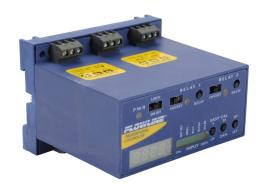
Flowline DataPoint remote level controller, tank fill or drain and alarm, 4-20 mA level sensor input, (1) SPDT non-latching relay, (1) SPDT latching relay, adjustable time delay, 4-20 mA repeater output, 120/240 VAC operating voltage.
