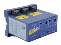
Flowline Switch-Pro remote level controller, tank fill or drain and alarm, (3) level switch input, (1) SPDT non-latching relay, (1) SPDT latching relay, adjustable time delay output, 120/240 VAC operating voltage.
