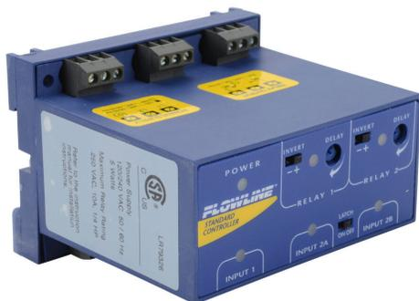
Flowline Switch-Pro remote level controller, tank fill or drain and alarm, (3) level switch input, (1) SPDT non-latching relay, (1) SPDT latching relay, adjustable time delay output, 120/240 VAC operating voltage.
