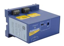
Flowline Switch-Pro remote level controller, tank fill, drain or alarm, (1) level switch input, (1) SPDT non-latching relay, adjustable time delay output, 120/240 VAC operating voltage.
