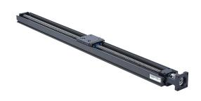
SureMotion linear actuator assembly, Gen 2 value, 2.360in wide, 24in travel, lead screw, 0.5in pitch, hard coated aluminum rail.
