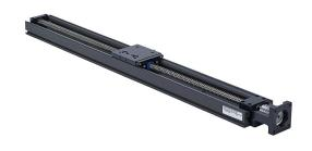
SureMotion linear actuator assembly, Gen 2 value, 2.360in wide, 18in travel, lead screw, 0.5in pitch, hard coated aluminum rail.
