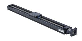
SureMotion linear actuator assembly, Gen 2 value, 2.360in wide, 18in travel, lead screw, 0.2in pitch, hard coated aluminum rail.
