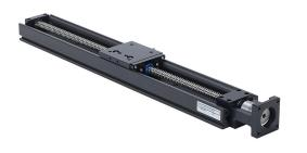
SureMotion linear actuator assembly, Gen 2 value, 2.360in wide, 12in travel, lead screw, 0.5in pitch, hard coated aluminum rail.
