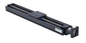
SureMotion linear actuator assembly, Gen 2 value, 2.360in wide, 12in travel, lead screw, 0.2in pitch, hard coated aluminum rail.
