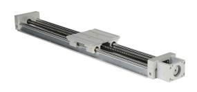
SureMotion linear actuator assembly, twin round shaft, 5.500in wide, 24in travel, ball screw, 0.2in pitch, carbon steel rail.
