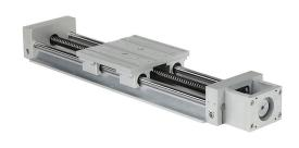
SureMotion linear actuator assembly, twin round shaft, 5.500in wide, 12in travel, ball screw, 0.2in pitch, carbon steel rail.
