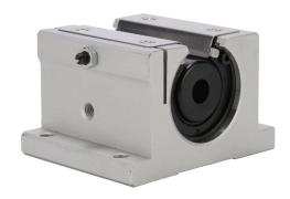
SureMotion single pillow block, linear ball bearing, 2.63in overall length, 1in inside diameter, aluminum housing. For use with 1in diameter SureMotion shafts.
