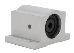
SureMotion single pillow block, linear ball bearing, 2.06in overall length, 3/4in inside diameter, aluminum housing. For use with 3/4in diameter SureMotion shafts.
