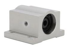
SureMotion single pillow block, linear ball bearing, 1.69in overall length, 1/2in inside diameter, aluminum housing. For use with 1/2in diameter SureMotion shafts.
