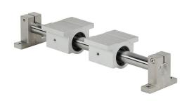
SureMotion slide element, end supported, round shaft, 3/4in shaft diameter, 12in overall length, carbon steel. (2) single pillow blocks included.
