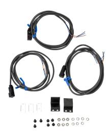
SureMotion inductive proximity sensor, rectangular, 8 x 7.4 x 17mm, polyarylate resin housing, top sensing, PNP, (2) N.C./(1) N.O. outputs, 2.5mm sensing distance, 1 kHz switching frequency, IP67, pigtail. Package of 3.
